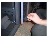
3. Offer up the second fixing plate to bottom bracket
