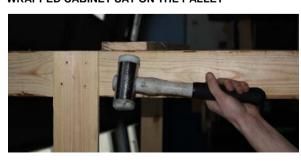
WHILE CABINET IS STILL ON THE PALLET, REMOVE ALL THE PACKAGING & BUBBLE WRAP AND THEN PROCEED TO REMOVE THE FRONT AND REAR DOORS PLUS THE SIDE PANELS TO ALLIEVIATE THE WEIGHT OF THE CABINET WHEN REMOVING FROM PALLET.
