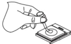
Apply thermal grease on CPU
