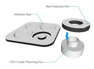
With the motherboard turned upside down, located the CPU cooler mounting holes. The hole position will vary depending on the brand and model of CPU. Peel the protective film from the adhesive pads and stick the nuts to the underside of the motherboard ensuring they correctly align with the holes. The slightly raised rim of the nut should fit through the motherboard CPU mounting holes.
