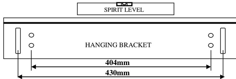
**Step 2:** Locate wall box onto hanging bracket. Mark out and drill hanging positions
